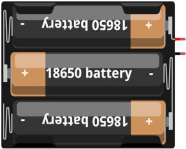
3 x 3.7 V Batteries
